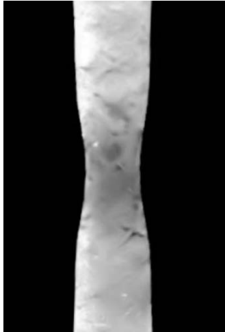
Fig. 9. X-ray radiography of a POM sample deformed in uniaxial tension at 160 °C with a strain rate of 10^{-3} \text{ s}^{-1} (the maximum true strain was \epsilon_{33} = 1.2 ).
